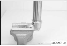
Take out the fork leg and clamp with the axle clamp.
