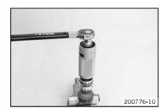
Align both pistons using the special tool.
