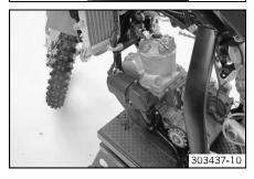
Lift out the engine from the side.
