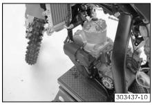
Position the engine in the frame.
