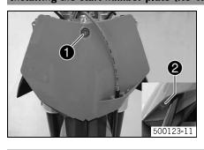
Position the start number plate. Mount and tighten screw ①.
