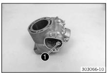
Remove screw • with the bushing and spring.
