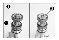
Disassemble the damper. (\* p. 42)
