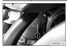
The shock absorber part number  $oldsymbol{0}$  is stamped on the top of the shock absorber above the adjusting ring on the engine side.
