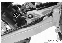
Remove shaft seal rings 3 on both sides.
