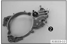
Mount adjusting spring ② with the auxiliary spring and spring insert.
