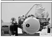
Position the kick starter. Mount and tighten screw ①.
