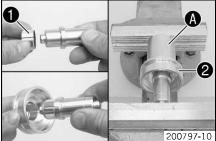
Slide the new pilot bushing • onto the special tool.
