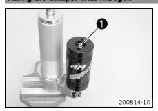
Screw in the screw • approx. two turns, but do not tighten.
