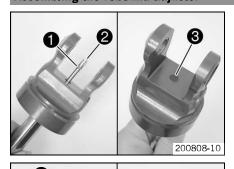
Grease O-ring • of the rebound needle.
