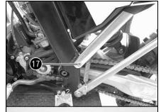
Remove the fixation and position the subframe.
