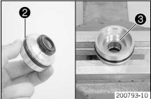
Grease the O-ring groove.
