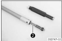
Remove piston rod 2 from the cartridge.
