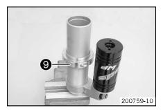
Remove adjusting ring 9 with the intermediate washer.
