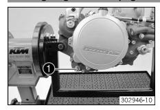
Mount and tighten the gear oil drain plug • with the magnet and the new seal ring.
