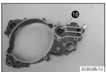
Remove shaft seal ring •.
