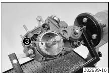
Mount special tool **3**, apply counterpressure, and pull off the rotor by screwing in the screw.
