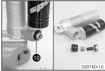
Remove compression adjuster •. Remove the spring and piston.
